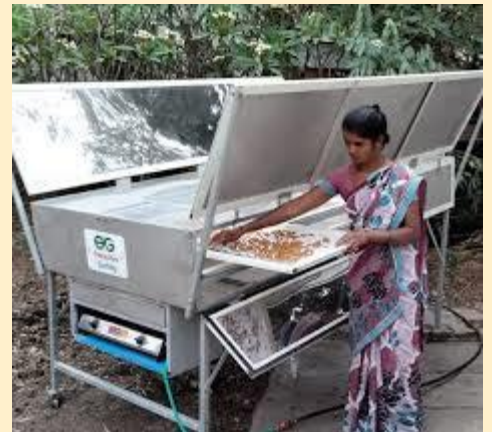
SOLAR DRYER at custom temperature using IoT based controller
